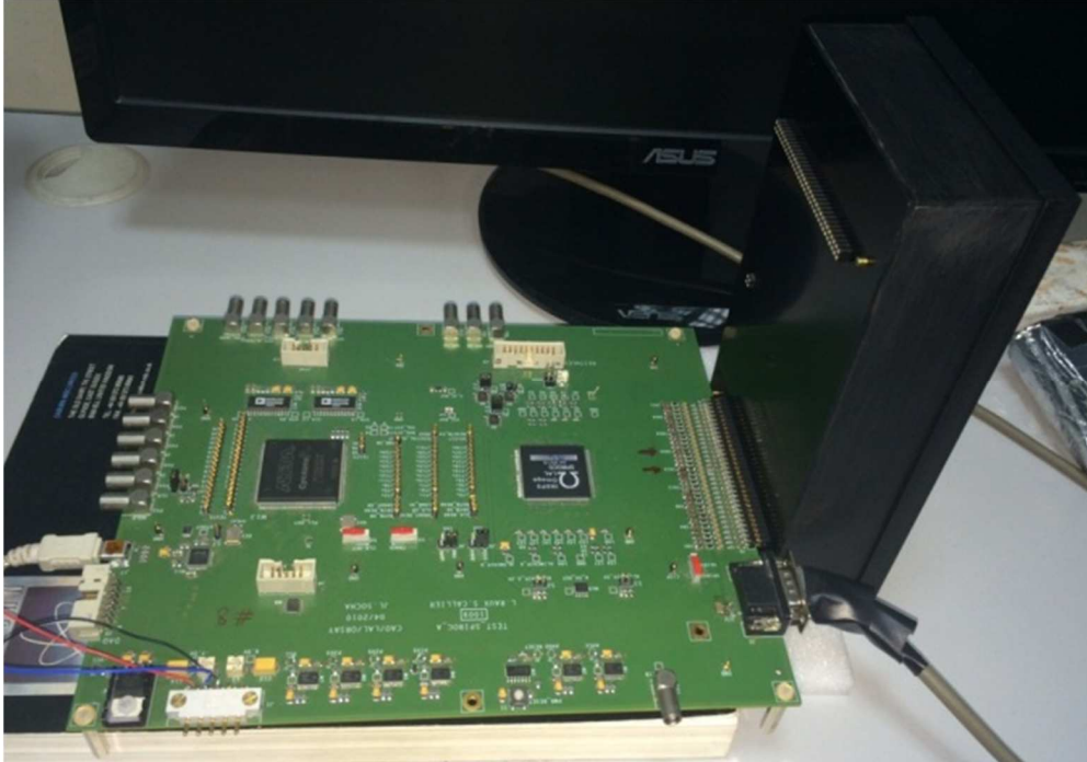
Fig. 22. Complete experimental apparatus for SiPM characterization.
