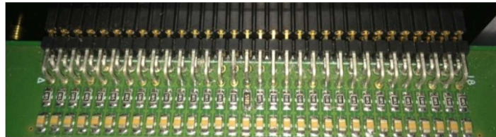
Fig. 13. SiPM board connection to the EASIROC evaluation board through the strip connectors.
